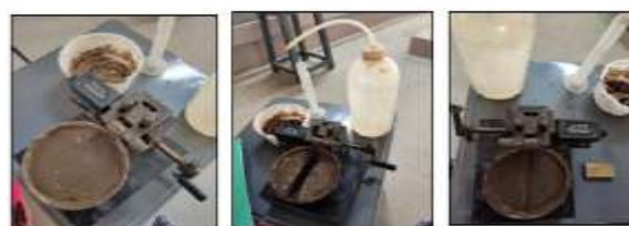
Fig 12. Liquid Limit Apparatus
