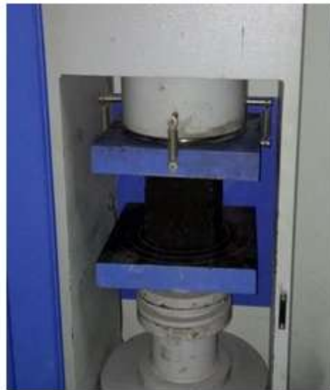
Figure3.Compressive strength test of cube using CTM
