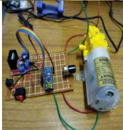
Figure 6: The water speed control of submersible water pump by aurdino
