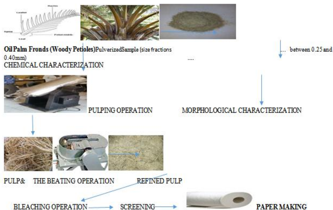
Figure 1: Steps in Oil Palm Fronds (Woody Petioles) fractionation and conversion to paper
