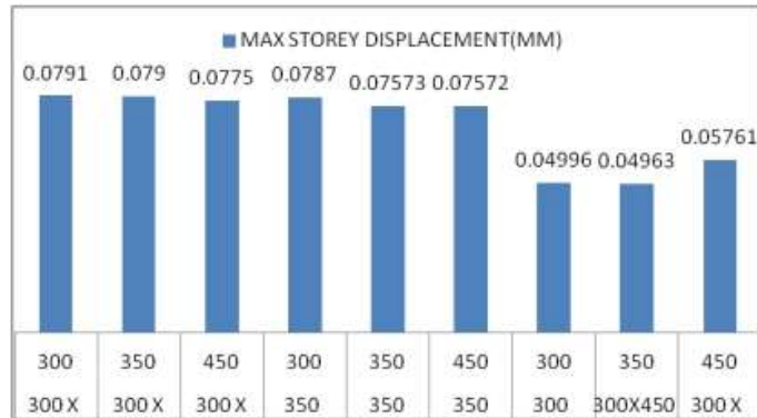
Graph -7: Result of Max Storey Displacement for Hybrid / Composite Structure by inserting Rectangular / Square Tubular Beam and Circular Tubular Column
