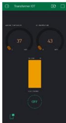
Figure 8 Load control – OFF state
