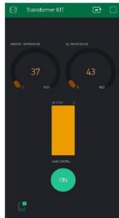
Figure 7 Load control – ON state
