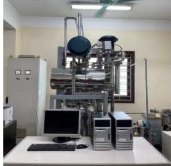
Figure 8: Experimental structure of boiler level control
