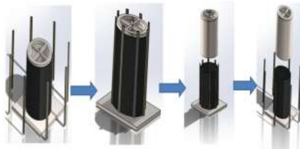
Figure 3.6 a- Eight Jaws moving towards the mould and sleeve
