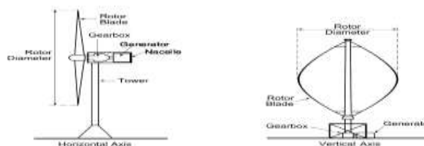
Fig 1: Horizontal and vertical axis type of wind turbines
