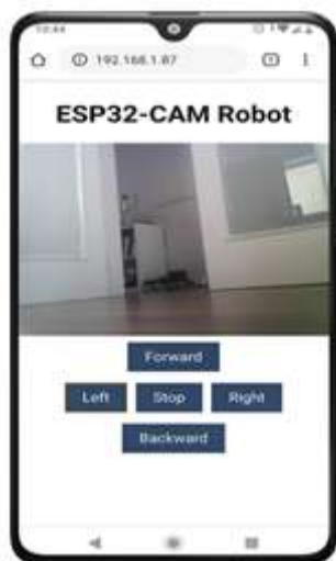
Fig 5: ESP32 Cam with live video streaming
