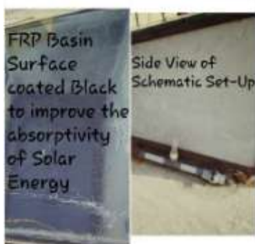
Fig. 4 Top View depicting the Black Paint coating on the Surface of Basin
