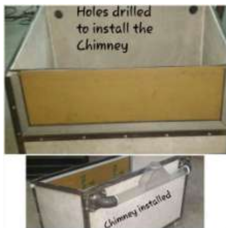
Fig.5 Holes drilled in the Rear Wall of the Still & Chimney installed in it.
