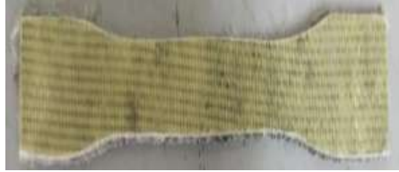
Fig 3: The specimen sample prepared in dog bone shaped for experimental analysis.
