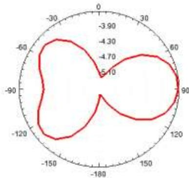
**Figure 8.** Azimuthal pattern (H-plane) gain plot (for  $\phi = \text{all values}$  and  $\theta = 90\text{degree}$ )
