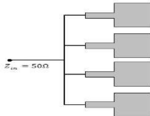
**Figure 3.** Four element micro strip array
