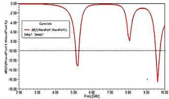
**Figure 5b.** Return loss graph for dual band antenna
