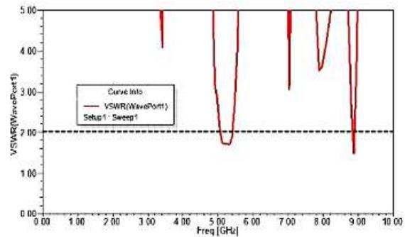
**Figure 10.**VSWR plot for the dual band array antenna
