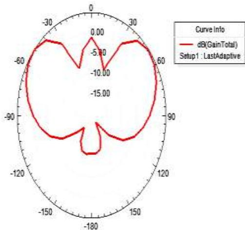
Figure 11. Elevation pattern (E-Plane) gain plot (for  $\theta = \text{all}$  values and  $\phi = 0 \text{ degree}$ )
