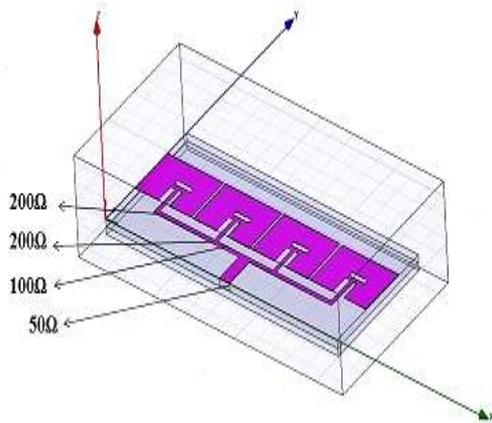
**Figure 4.** Simulated dual band array antenna design
