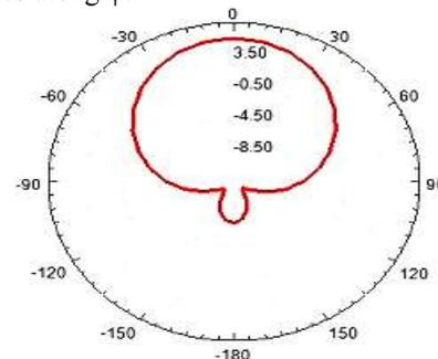
**Figure7.** Elevation pattern (E-Plane) gain plot (for  $\theta=all$  values and  $\phi = 0$ degree)
