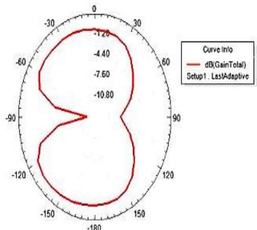
Figure 12. Azimuthal Pattern (H-plane) gain plot (for  $\phi = \text{all}$  values and  $\theta = 90 \text{ degree}$ )
