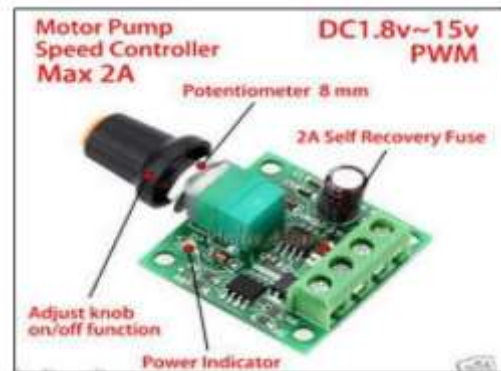
Figure No.5 – DC Motor PWM Speed Regulator 1.8V, 3V, 5V, 6V, 12V-2A speed control switch
