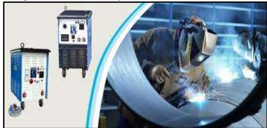
Figure No.1– Co2 Welding For Circular Pipes
