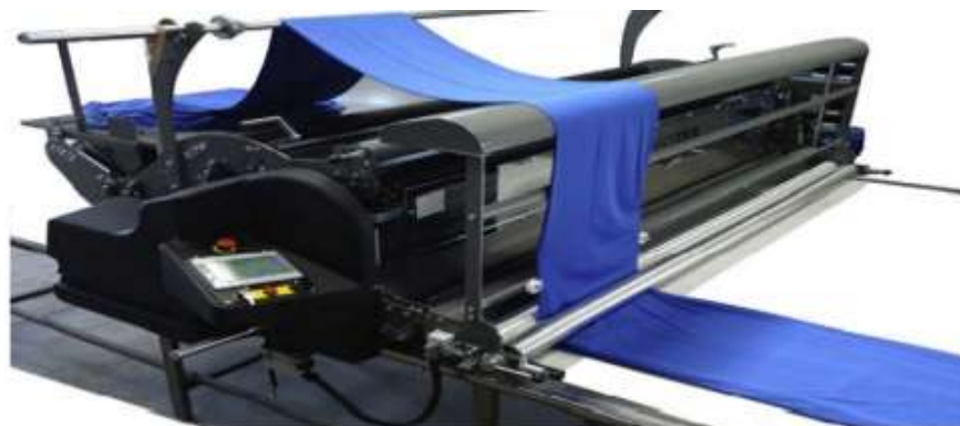
Figure 7. The automatic spreading machine Apolo Smart 300 by Cosmotex equipped with several special devices to lay tubular fabrics.
