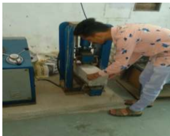
Fig.5. Flexural Strength of Polymer Concrete At 28 Days
