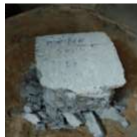
Fig.3. Compressive Strength test of cube.
