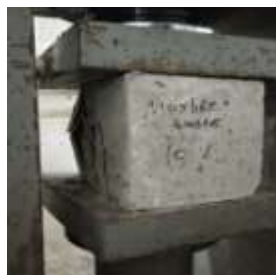
Fig.3. Compressive Strength test of cube.
