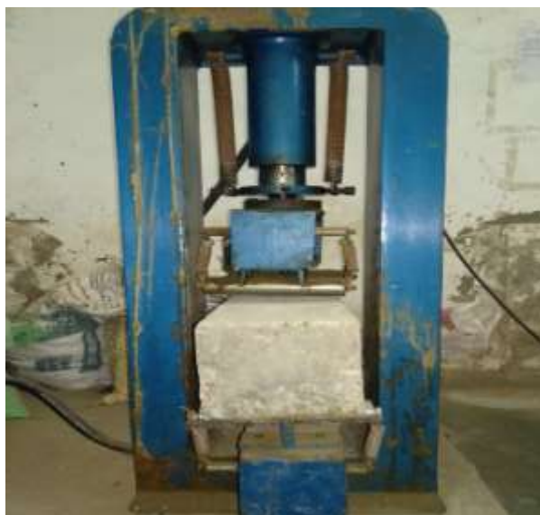
Fig.6.Flexural strength test of beam.
