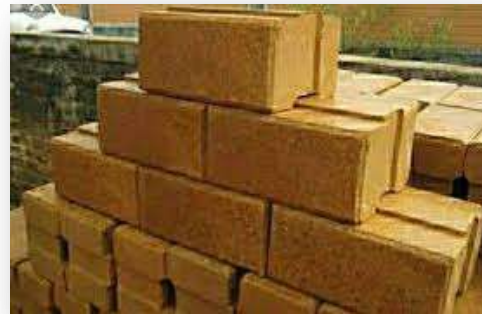
Fig.[12] Picture showing Mud Concrete Blocks [71]
