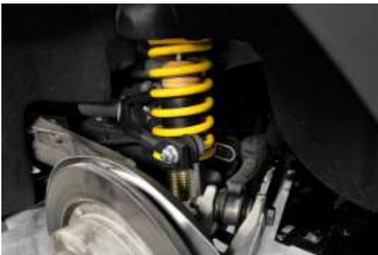
Rear suspension used in scorio is MULTI-LINK COIL SPRINGS SUSPENSION WITH ANTI-ROLL BAR.
